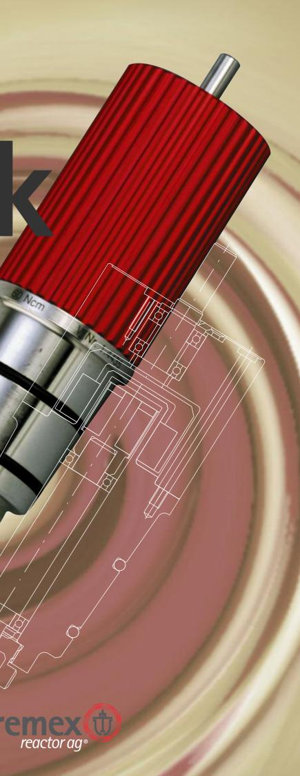
The magnetic stirring action of mrk2 «alluro»: Power is transmitted from the stirrer motor to the drive collar by means of a flexible coupling. The drive collar is fitted with a magnetic ring, which uses the mutual attraction of the magnetic fields to couple with the inner magnet. This means that the stirrer shaft is driven without any contact.
